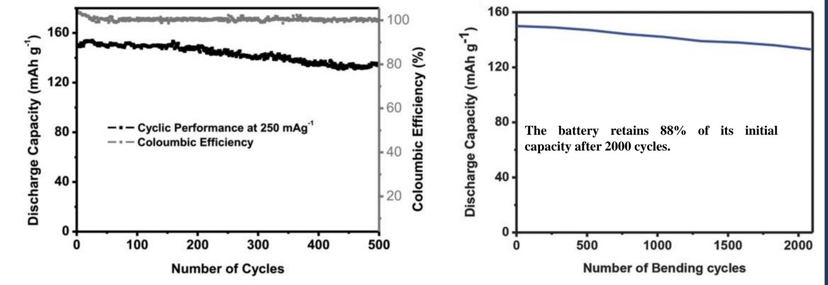
A sulfur-linked carbonyl-based poly(2,5-dihydroxyl-1,4-benzoquinonyl sulfide) (PDHBQS) compound was synthesized and used as cathode material for lithium-ion batteries (LIBs). Flexible binder-free composite cathode with single-wall carbon nanotubes (PDHBQS–SWCNTs) was then fabricated through vacuum filtration method with SWCNTs.
